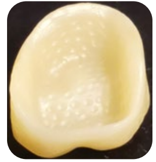
"Pockmarks" as produced by the lab pre-sintering
