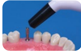
Magnetic pulses stimulate implant while device analyzes rigidity
